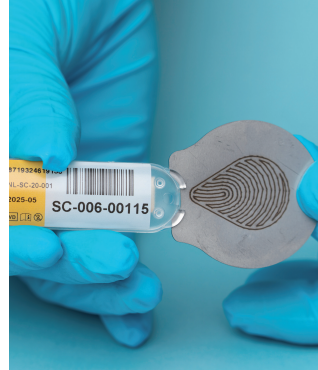
2. Open Ser-Col with the opener and remove the paper strip
