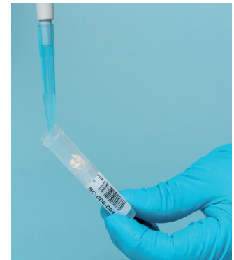
8. Add 100-150 \mu l elution buffer/cm serum paper, depending on the LOD of the analysis.
