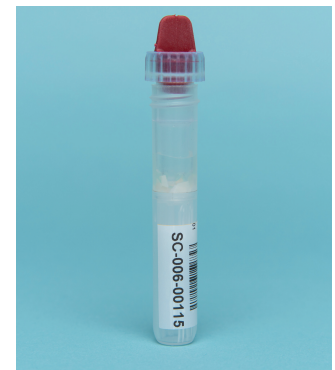
12. Close the tube with the separator cap until analysis
